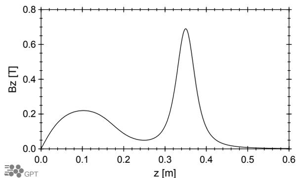
Figure 3: Magnetic field profile on-axis.
