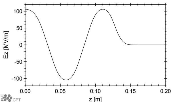
Figure 2: Electric field-profile on-axis.
