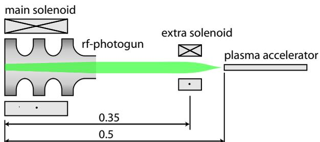
Figure 1: Schematic layout of the set-up.
