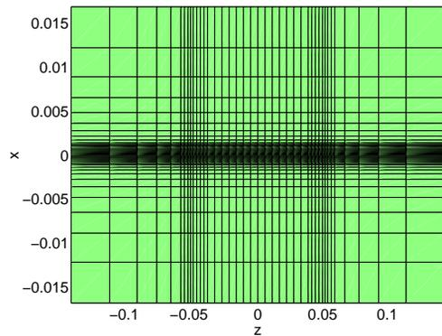
Figure 2: The discretization of a cigar shaped bunch (( $x, z$ )-plane): wavelet mesh with  $45 \times 45 \times 41$  mesh lines.
