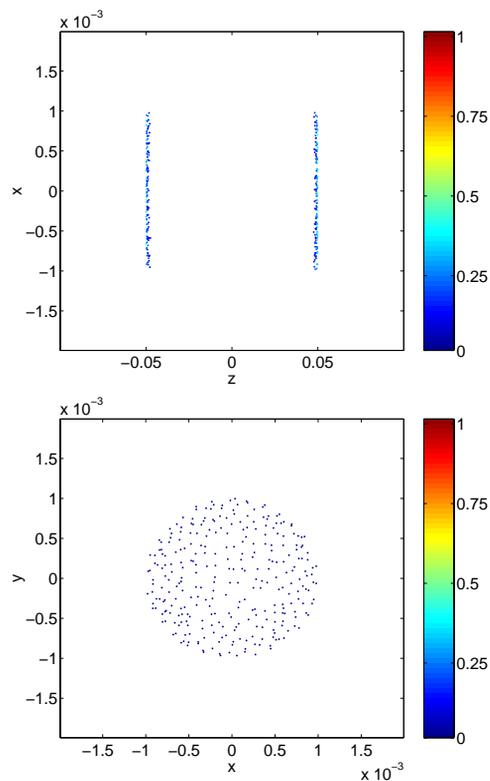
Figure 4: Cigar bunch with  $A = 0.01$ : Particles with relative error of the electrical field  $> 0.1$  for a wavelet mesh with  $45 \times 45 \times 41$  mesh lines. Transversal direction (top), longitudinal direction (bottom).
