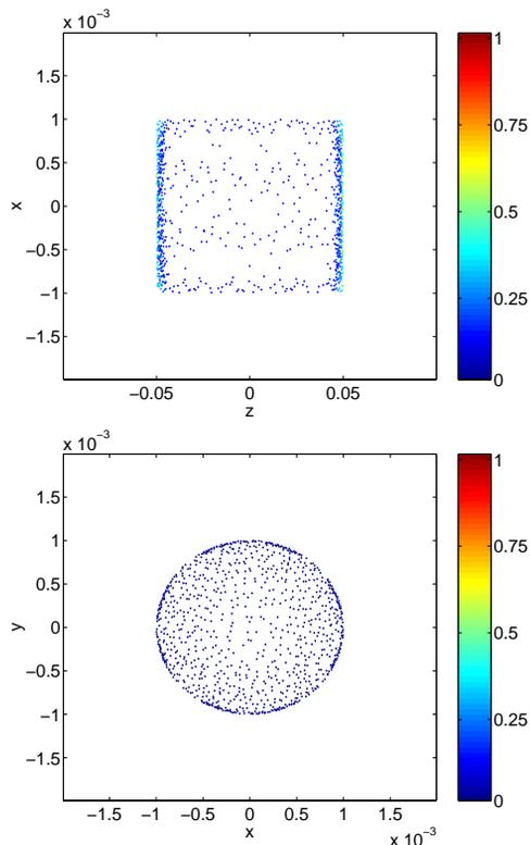
Figure 3: Cigar bunch with  $A = 0.01$ : Particles with relative error of the electrical field  $> 0.1$  for a  $33 \times 33 \times 33$  mesh. Transversal direction (top), longitudinal direction (bottom).
