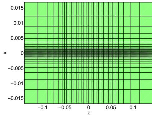
Figure 1: The discretization of a cigar shaped bunch (( $x, z$ )-plane): grid with  $33 \times 33 \times 33$  mesh lines distributed following the particle distribution.
