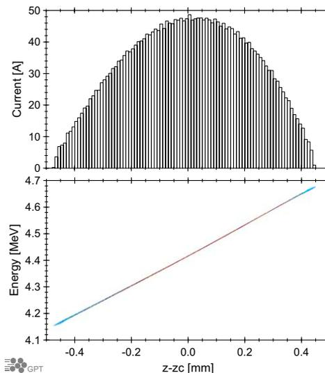
Figure 5: Current profile and the distribution in longitudinal phase space of the bunch 3 ns after initiation, corresponding to a centroid position  $z_c \approx 0.9 \text{ m}$ .
