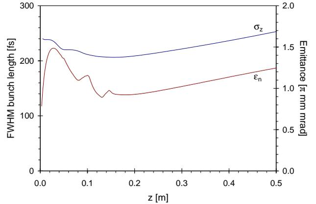
Figure 4: Bunch length and emittance evolution for a parallel beam.
